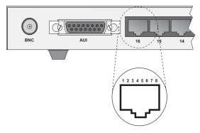
Fig. A-1 RJ-45 Connector Pin Numbers
